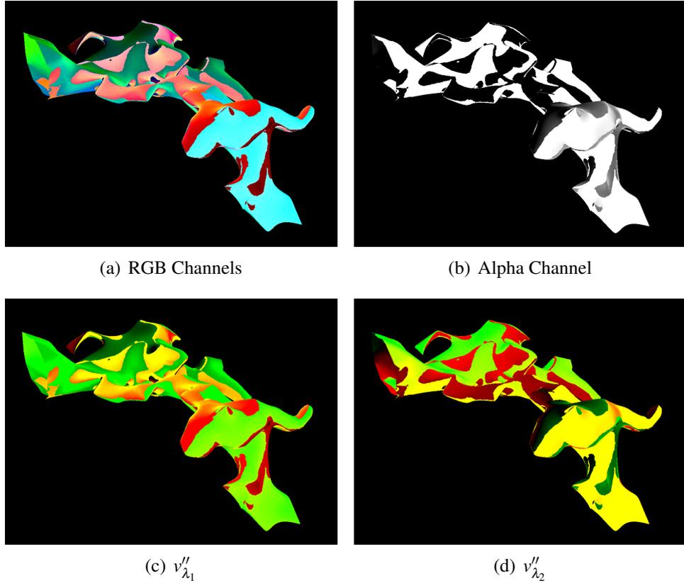
**Figure 4.2:** Both eigenvectors  $v''_{\lambda_1}$  and  $v''_{\lambda_2}$  scaled to  $[0, 1]$  and stored in red, green, blue and alpha channel of a texture (a and b). In addition, we separated both eigenvectors into two images, each showing the x and y component in the red and green color channel (c and d) for illustration.
