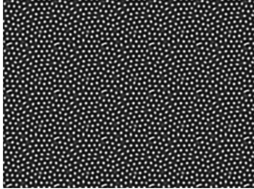
**Figure 4.3:** *Hundred per hundred pixel reaction diffusion texture created using Alan Turing's method. It got tiled to create a texture of required size, since reaction diffusion is computational expensive. Minor artifacts resulting from tiling can be seen, but ignored in practice due to the advection step.*
