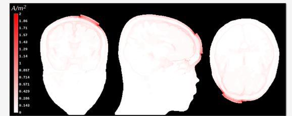
**Current density magnitude plot for tDCS example on cutting planes.** Although standard, slice-based visualizations suffer from missing spatial and directional information, which play an important role in electrical fields.
